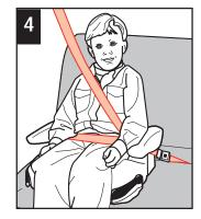
Place lap belt across child's thighs. Lock buckle. The belt should cross the base of the child's neck and across the chest (not the face or neck). Pull up on the shoulder belt to tighten. NOTE: Make sure the
